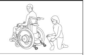
Before using the wheelchair each day, check the residual capacity of the battery. If the residual capacity of the battery is low, the battery may run out during operation and it may become impossible to travel in power drive mode.
