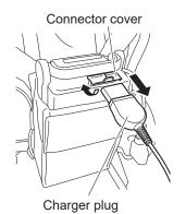
⑤ Check that the charge lamp (green) on the charger turns on.
