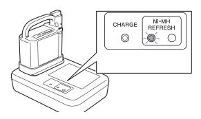
In a refresh charging process, after all remaining electricity has been discharged, the refresh lamp (orange) turns off. The charge lamp (green) comes on and a normal charging process begins. The time it takes from the start of refresh charging to the completion of normal charging is 3 – 19 hours.
