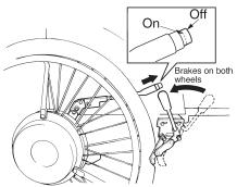
⑤ In the case of quick connector Align white-colored arrow mark on the cable side coupler with another white mark printed on the wheel side coupler (left or right wheel), insert the coupler until you hear clicking sound.
