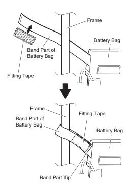
Case of Battery Bag Band Tip Part Reaching to Battery Bag
