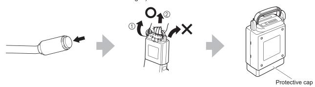
Please open the Battery-bag and take out the battery in the same manners as that of Ni-MH Nickel Metal Hydride Battery.
