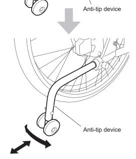
Check that the safety wheels on the ends of the anti-tip devices are 35-50 mm (1.4-2.0 inches) above the ground when the casters and rear wheels are in contact with the ground.
