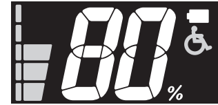
Battery residual capacity indication
