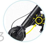
Take the pull device and insert the docking pin ends into the central bracket of the subframe.
