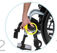
Now rotate the tommy screws of the clamps in a clockwise direction until they are hand tight and the intermediate sub-frame is securely held in the clamps.
