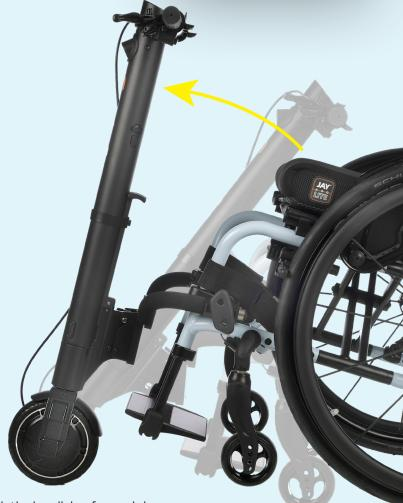
Push the handlebar forwards/ upwards until the locking bolt automatically clicks into place. Only release the wheelchair brakes once device is locked in place.
