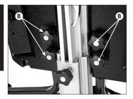
The tray angle can be adjusted by loosening the plastic handle **()** on either side of the tray, set the tray to the required angle and tighten the plastic handles again securely.
