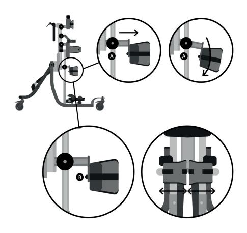
The headrest should only be used when the child is in supine standing. To adjust the height, depth and angle of the contoured headrest, loosen the hand knobs and when set to the desired position re-tighten the knobs.
