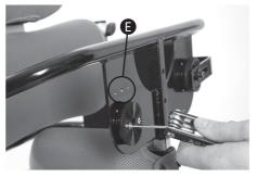
To attach the pommel, loosen the receiver allen bolt **©**, slide the pommel into the receiver **D** and tighten at the required depth. The height can also be adjusted using the allen bolt **©** at the back of the pommel.
