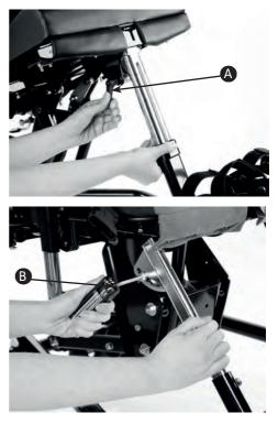
The footplate angle can also be adjusted for dorsiflexion and plantarflexion. To adjust for dorsiflexion, insert your Allen key in to the bolt below the footplate, directly in the centre, and turn right. To adjust for plantarflexion perform the same instructions but turn left.
