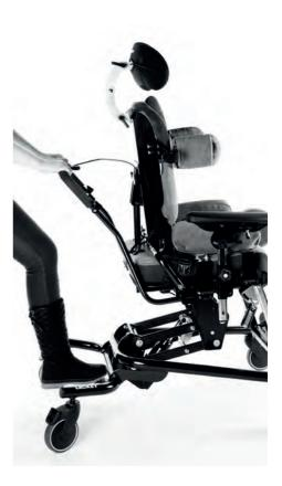
You can carry out this adjustment with the user in the chair. To adjust the height of the hi-low chassis use a pump action on the foot lever at the rear of the chassis whilst holding the push handle. Once you remove your foot from the pedal the seat will be fixed at the chosen height.
