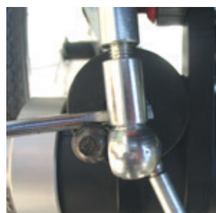
Remove the ball point by levering up the hinge using an appropriate tool.
