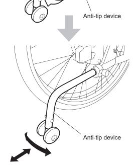
Check that the safety wheels on the ends of the anti-tip devices are 35-50 mm (1.4-2.0 inches) above the ground when the casters and rear wheels are in contact with the ground.
