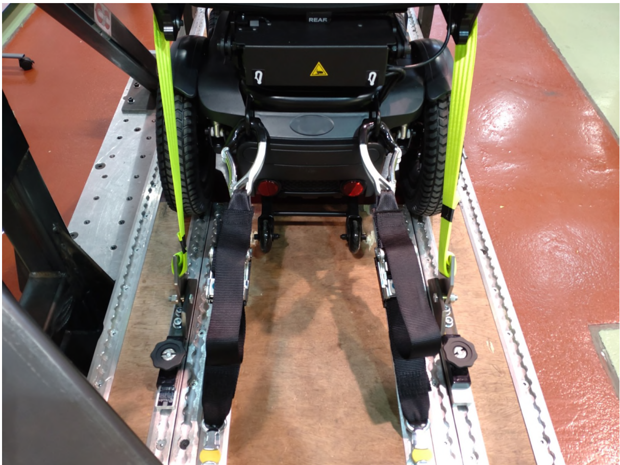
Figure 6: Rear tie-downs, pre-test
