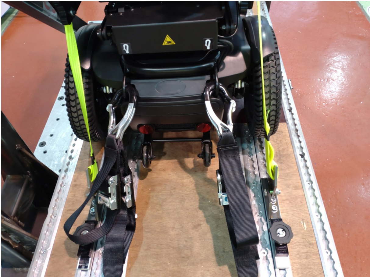
Figure 14: Rear tie-downs, post-test
