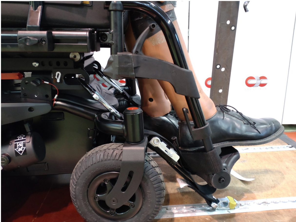
Figure 16: Front tie-downs, post-test
