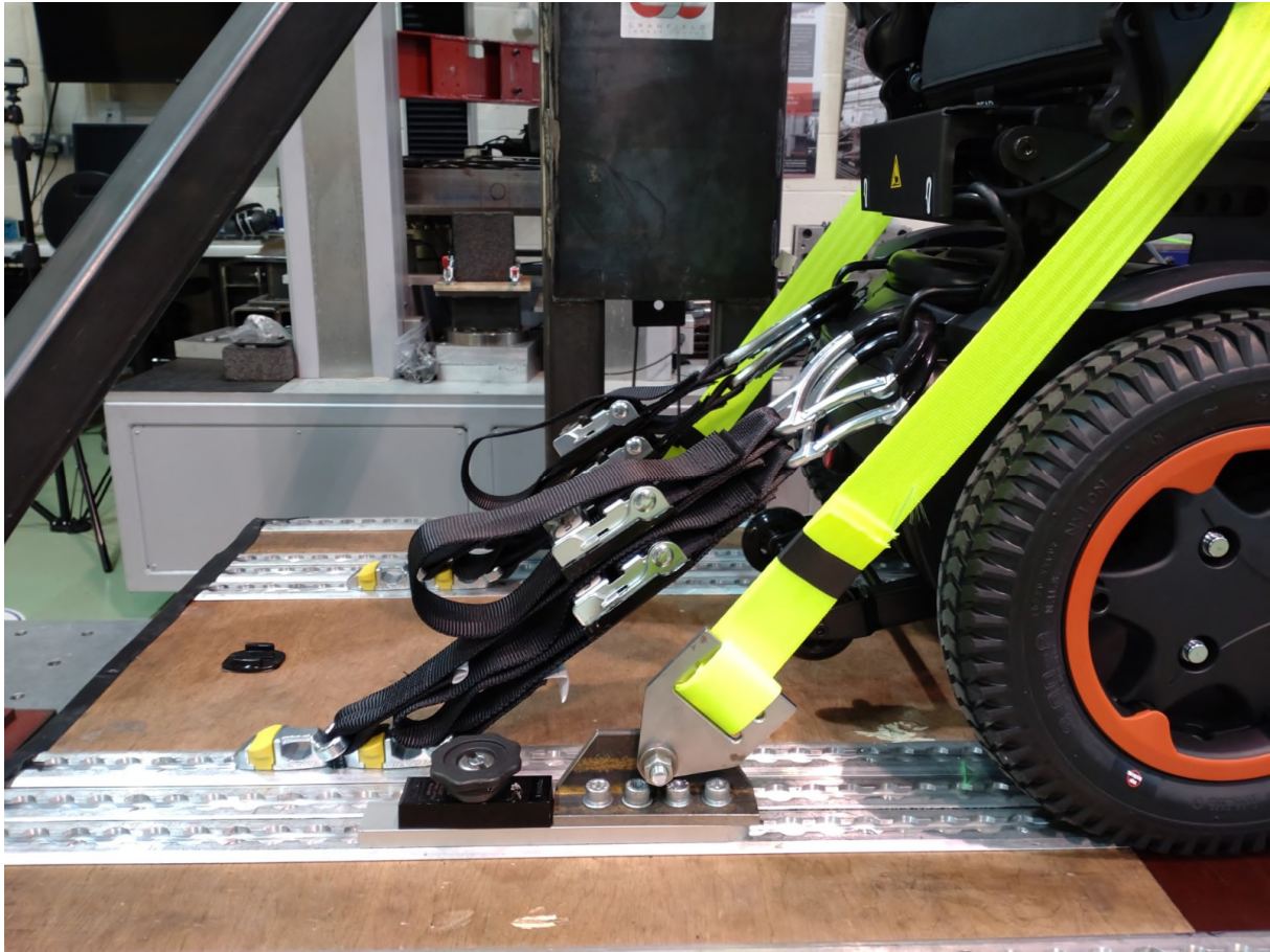
Figure 7: Rear tie-downs, pre-test
