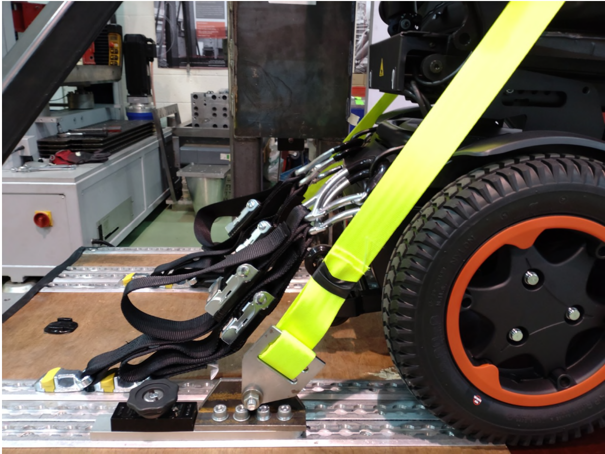
Figure 15: Rear tie-downs, post-test
