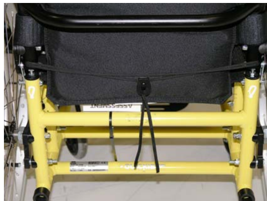
Position of the rear wheelchair tie down restraint and the tie down label on the wheelchair.
