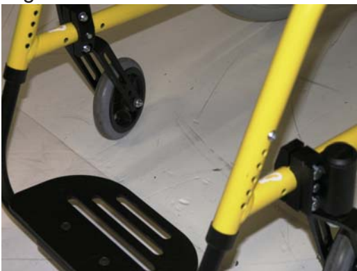
Position of the front wheelchair tie down restraint and the tie down label.
