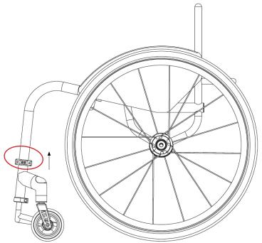
Finally move the clamps up the seat rail an extra 5mm and tighten up the bolts, this gives the FrontWheel an extra tight fit.
