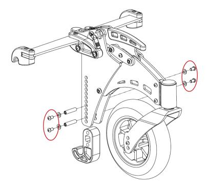
To do this simply remove the highlighted bolts from the FrontWheel and slide out the axles. This then allows the footrest hook to be removed and moved to the correct position. See illustration to the left.
