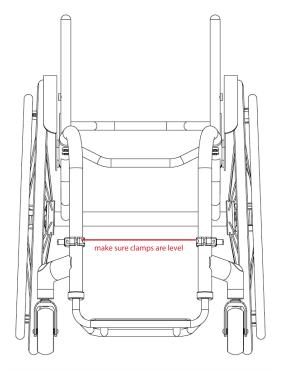
Locate the clamps so that the polished steel lugs face out and nip up so that you can still move them up or down the seatrail.
