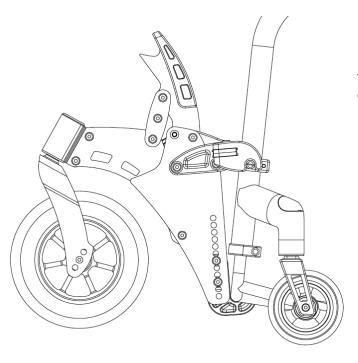
To lock the FrontWheel in place, press the clamp handle down until it touches the hook plate.
