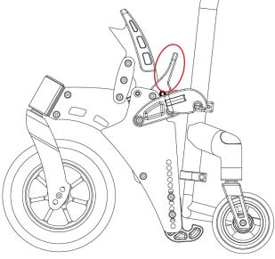
Now remove the FrontWheel, to do this lift the clamp handle.
