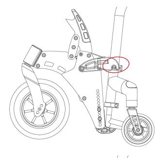
Next lock the FrontWheel in the up position and locate the footrest hook under your footrest. Now adjust the positions of the clamps up the seatrail so that the FrontWheel is tight around your footrest and around the steel lugs as illustrated to the left.
