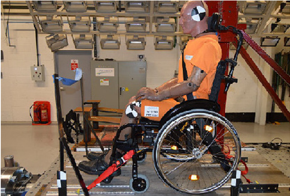
Wheelchair secured on the rails, before impact
