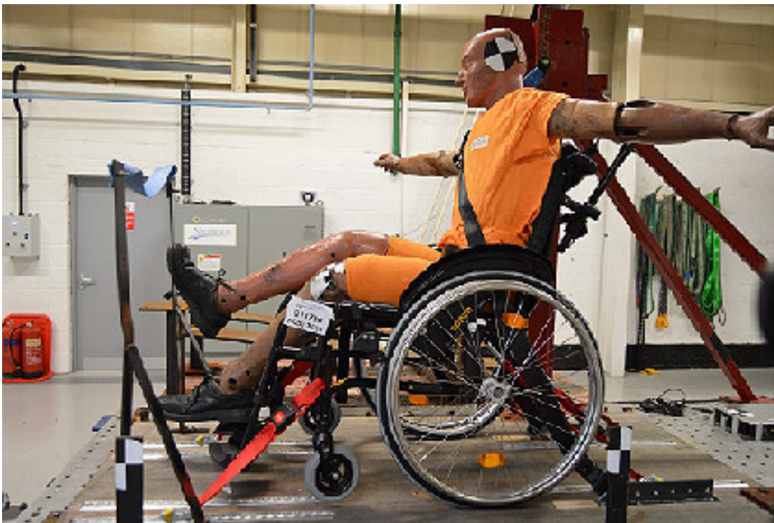
Wheelchair secured on the rails, after impact
