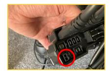
2. The new VR2 PM2 power module has an additional connector attached that has NO function.
