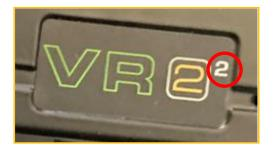
1. The new VR2 PM2 hardware can be identified with the label having the additional number attached:
