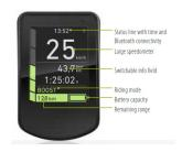
// Cc nnect Display cc nnects with your smartphone (download of neodrives app necessary) Records trip data such as average speed, maximum speed, trip distance, and total distance.
