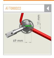
// ATTITUDE Manual with Standard fork: crank position range (adjustment via spacers in the upper docking clamp)
