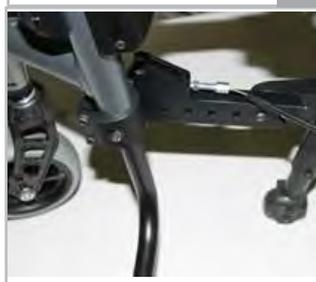
// To move the pedal position 2 cm closer or up to 6 cm further
