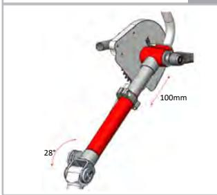
// ATTITUDE Manual / Hybrid - crank position range with option ATT080035 "Fork, angle and depth-adjustability of crank-position "
