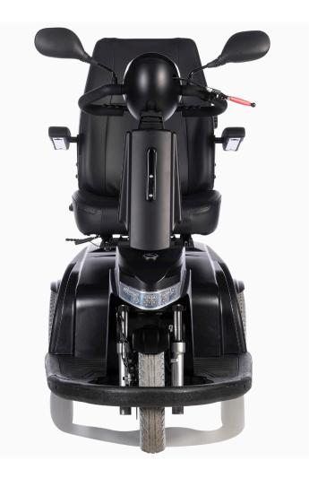
Front bumper as standard to reduce damage (for Elite² Mini)
