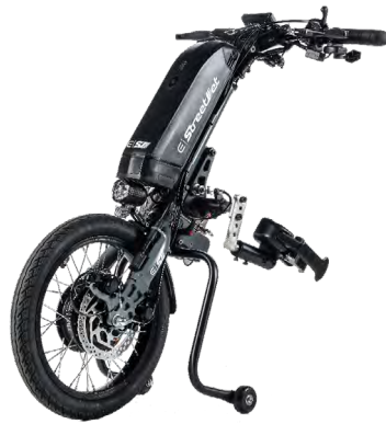
// STE070093 16 Inch wheel, pneumatic hybrid tyre, 250W/750W
