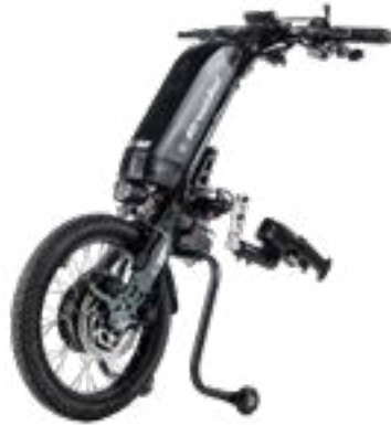
// STE070093 16 Inch wheel, pneumatic hybrid tyre, 250W/750W
