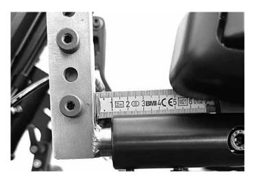
Ensure that there is in any case, no contact between the driving wheel/ stand and the footboard/ feet. (see section 5.0)
