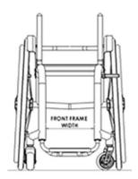
There are three different front frame width ranges available to fit your individual wheelchair measurements. Measured from inside tube to inside tube.
