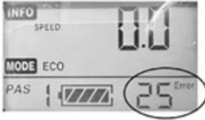
The fault code is always shown in the bottom right corner of the display.
