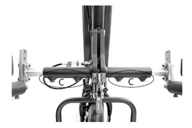
Make sure that the distance between mounting plate and clamp does not exceed 20mm.
