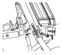
Tighten the screws (A) to 12Nm and (B) to 20Nm
