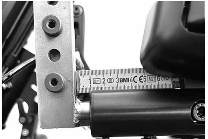
Ensure that there is in any case, no contact between the driving wheel/ stand and the footboard/ feet. (see section 5.0)
