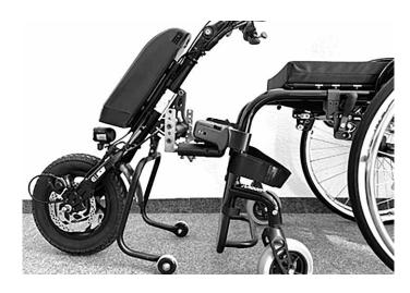
Close the clamps by pushing on the lever
