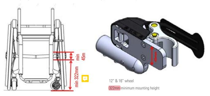
5 - Front Frame Width Measurement - The width of the front frame measured inside tube to inside tube on the minimum mounting height or above needs to be between 220mm - 425mm.
