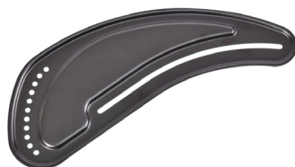
Aluminium sideguard, wet weatherprotection (in frame colour)
