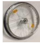
Rear wheel, drum brakes, 36 spokes, cross-wise spokes
