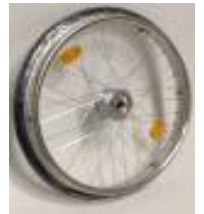
Rear wheel, drum brakes, 36 spokes, cross- wise spokes
