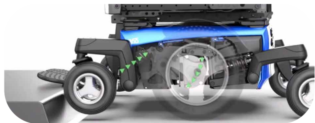
Step 1: The castor arm raises and forces the drive wheel into the ground, maximising traction
