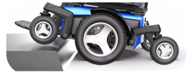
Step 3: The chair rocks onto the rear castor with the front castor elevated, allowing obstacle climbing
