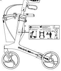
This label is placed on the inside right of the sideframe
