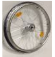
Rear wheel, drum brakes, 36 spokes, cross-wise spokes
