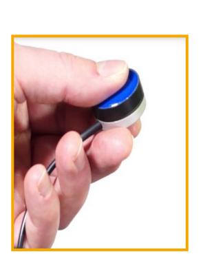
**Step 2:** Connect the R-Net Dongle. Open the PG programmer and read out the program.
