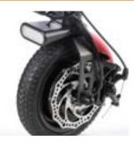
LED-light, Fender (accent colour red) and disc-brake (pictured on EMF070085 Drive wheel 8,5", solid tyre)
