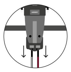
• If the frame is at a low height and the pulley straps are hanging down, you can attach them to the clips at the bottom of the framethis ensures the straps are out of the way.
