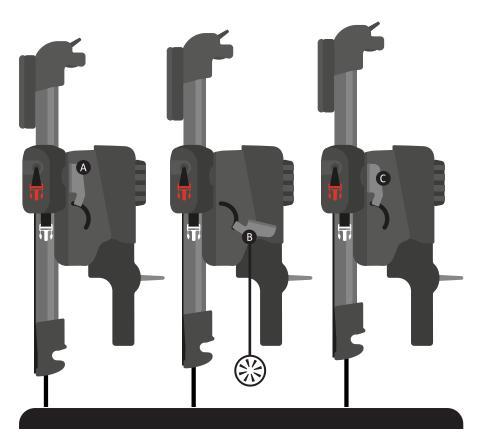
Note – fine height can only be used to increase height, it cannot be used to reduce height. Note – if you find adjustment of the fine height challenging, ask the user if they can support some of their weight if possible, or, ask another person to help and support some of the user's body weight.
