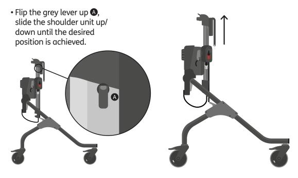
• Once the shoulder unit is in the desired position, flip the grey lever down again to lock.
