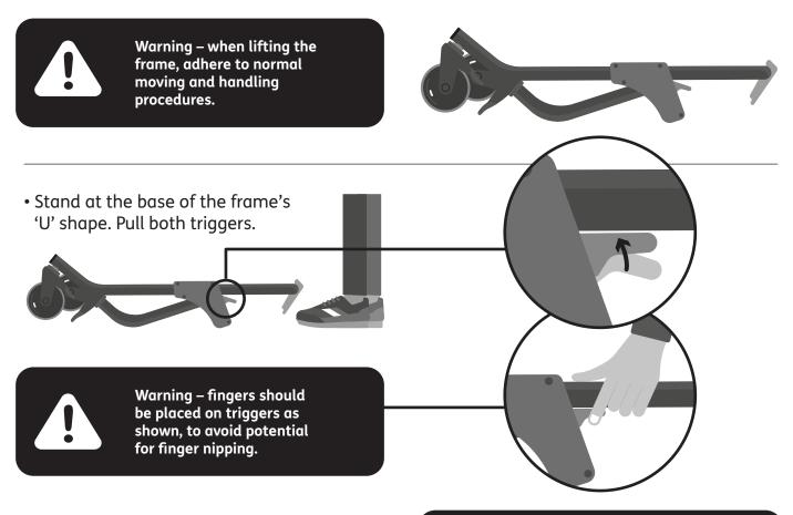
• Walk the frame's front legs forward, away from you (in direction of arrows), engaging the front castors until the legs are fully extended. Release both triggers.
