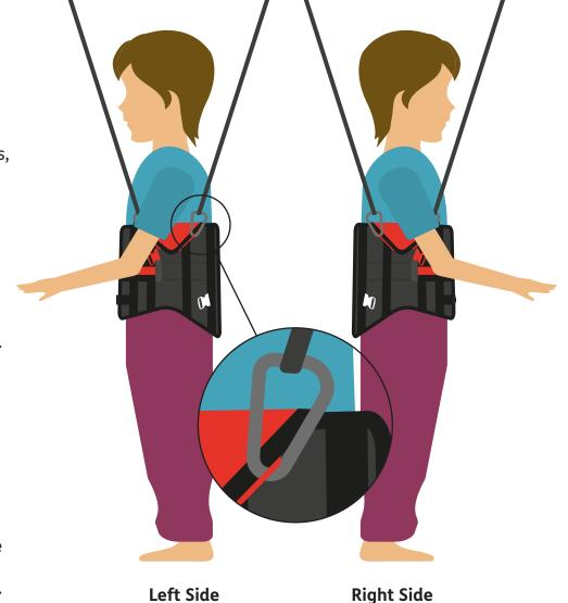
Warning – Always ensure both hoist straps are used. Never attempt to hoist using just one strap.
