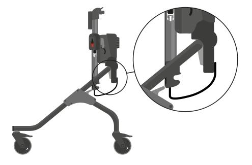
Warning – Only pull the pulley straps by placing hands in the loops- do not use feet.
