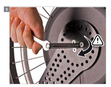
**Note!** When the axle is not properly secured in the motor, it may come loose!
