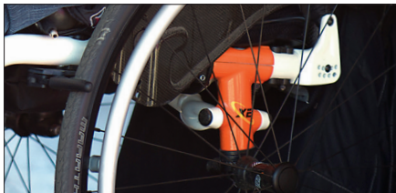
Centre of gravity adjustment in Orange (Xenon).
