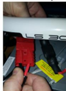
Remove the red and black battery shoe and pull them apart
