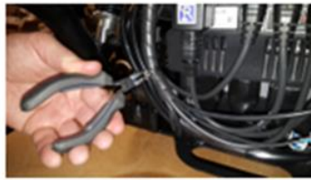
Cut the clips Carefully
