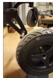
Loosen swivel wheel (rear)
