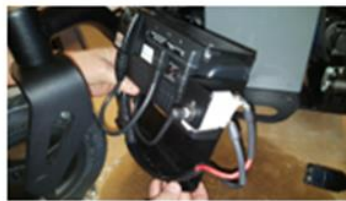
Lift Power Module aside.
