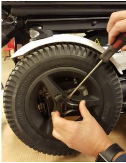
Remove cover with a screwdriver
