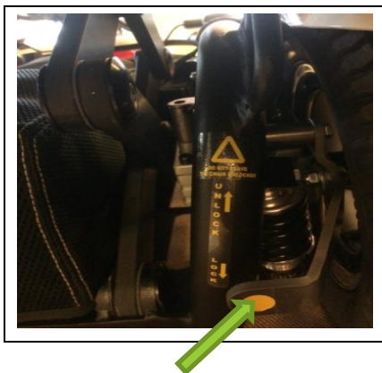
Lever for disconnect the motors
