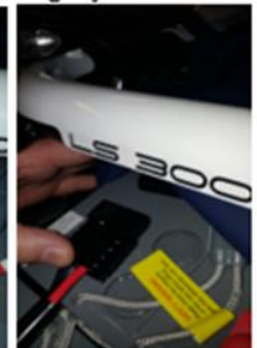
Remove the red and black battery shoe and pull them apart
