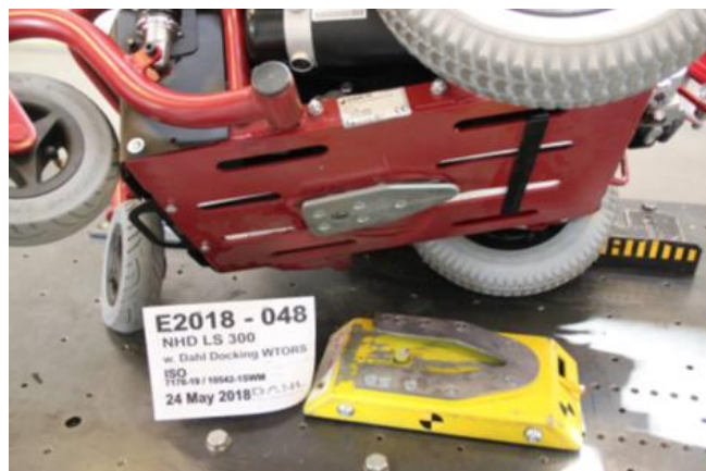
LS-300 shassis with Dahl Docking plate mounted
