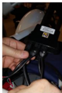
Lift away the light module
