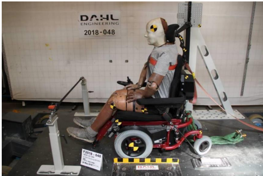
LS-300 crash test using Dahl docking station.
