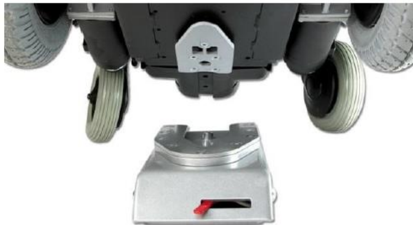
Docking station and docking plate on chassis
