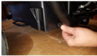
Unscrew the 4 finger screws
