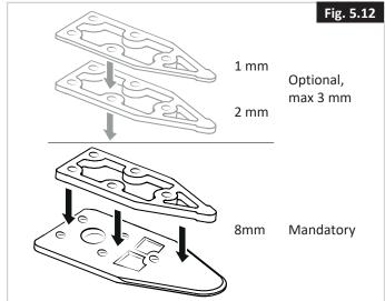
3. Put the five screws through the lock plate, the mandatory 8 mm spacer and the selected optional spacers (gray in picture) (Fig. 5.13).
