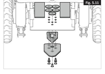
2. Use more spacers to achieve desired thickness with regards to, for instance, user weight and tire pressure. Additional spacers can be mounted under the locking station (Fig. 5.12). To align the height of the lock plate under wheelchair with the docking station fit spacers between the docking station and the vehicle floor to raise the docking station.
