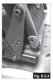
When assembled as shown in figure 8.2.2 it is possible to select 94 or 102° recline
