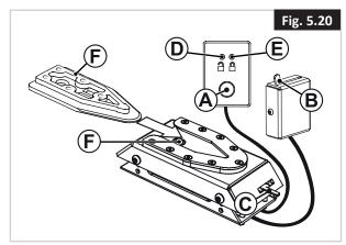
**WARNING!** Attempting to reverse the wheelchair before the red LED has been illuminated will result in blocking the docking stations lock mechanism, which makes it impossible to reverse. If this happens repeat above unlocking procedure.
