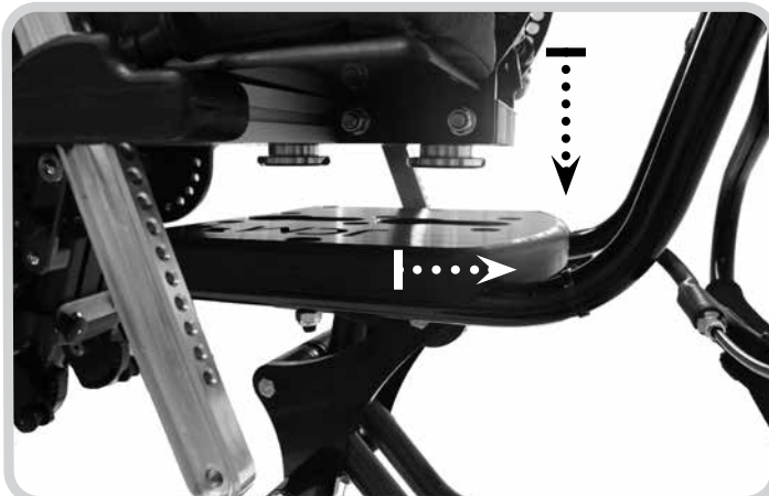
View from the side showing the seating unit lugs lowering into the interface plate cut outs.
