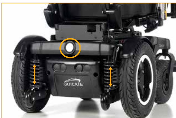
Full track suspension system.
