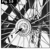
Hold the quick-release button on the axle depressed when inserting the axle into the frame to mount the rear wheels. Release the button to lock the wheel in place. The guick-release button should snap back to its original position.
