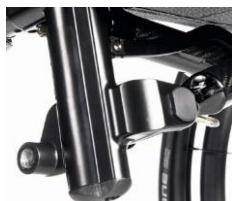
Axle-stems cut-to-length (KRF010412): specifically cut to your seat-height. Upwards adjustment limited (only +1 cm) (-200 g for rear seat height 430 mm compared to full-length axle-stem)
