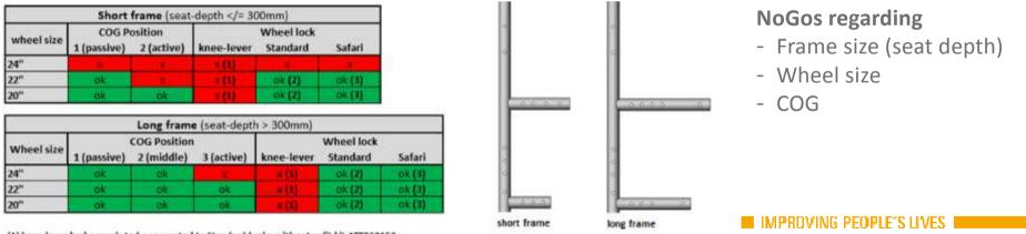
(1) knee-lever brake needs to be converted to Standard-brake with retro-fit kit ATT060150
