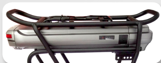
carrier battery (9Ah, 11Ah, 15Ah)
