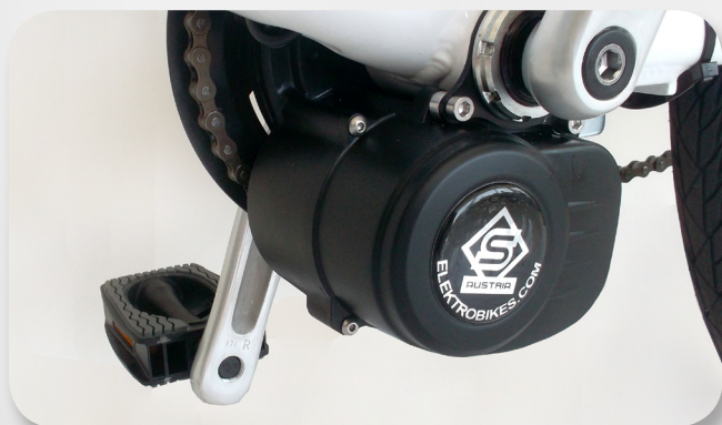
brushless center motor with integrated controller
