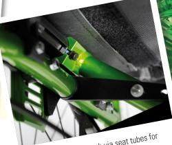
40 mm seat depth growth via seat tubes for growing user (without new parts).
