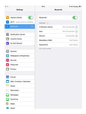
A list of devices will appear on the right side of the page. Select R-net iDevice Module. A successful pairing sequence will show the R-net iDevice Module as Connected.
