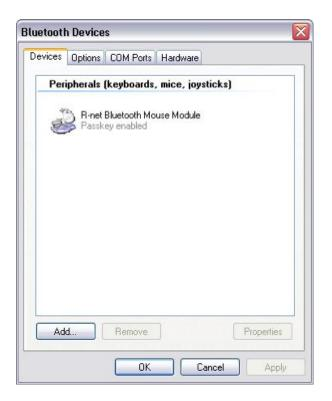
• If the process fails, click on 'R-net Bluetooth Mouse Module' and then 'Remove'. Repeat the procedure.
