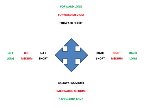
Parameters Short, Medium and Long Nudge Time set the interval for each joystick command (see Programming Chapter).
