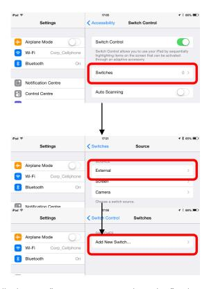
The iPad will ask you to "activate your external switch....". Select one of the R-Net commands, and deflect the joystick accordingly (**Short**, **Medium** or **Long** in the chosen direction).
