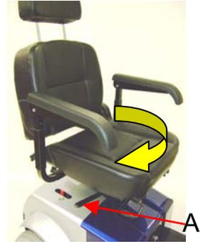
The armrest can be lifted and the seat can be swivelled to the side before mounting or dismounting.
