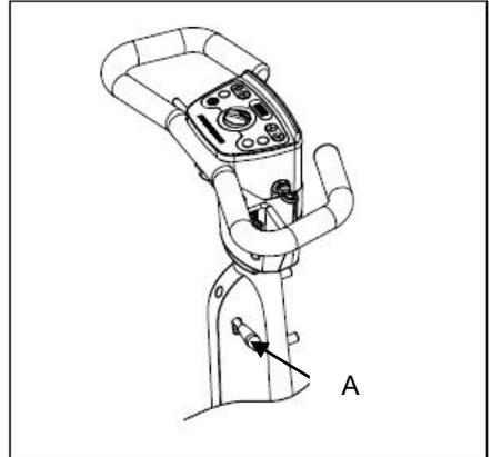
If you release the steering column while still pulling the handle down, the pneumatic spring will cause the steering column to jump into the most forward position automatically.
