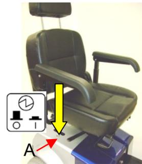
The automatic circuit breaker is located on the rear cover, under the seat.
