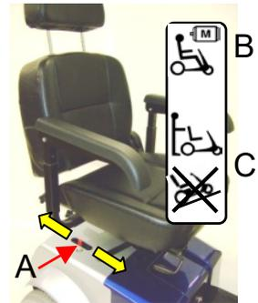
The Fortress Calypso's automatic parking brake can be reapplied by placing the neutral handle back into the BRAKE APPLIED position, (B).
