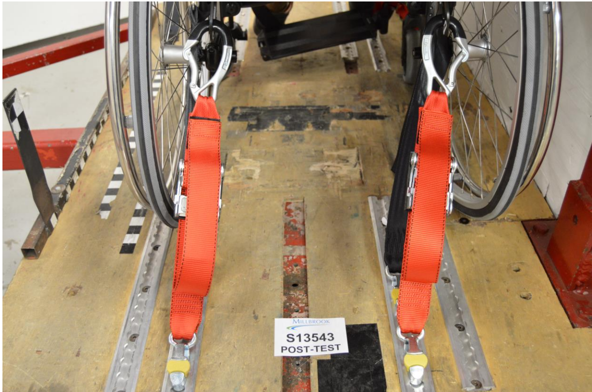
Rear wheelchair restraints, post-test
