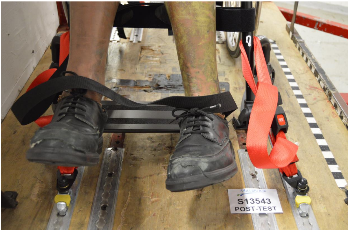
Front wheelchair restraints, post-test
