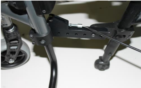
FMG-MA03-3201-01 Adaptation link -20 tot + 60 mm
