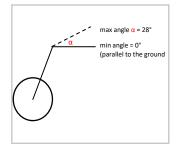
// Depth adjustability: 100mm (+/-50mm compared to standard fork) continuosly adjustable Angle adjustment: from 0° (parallel to the ground) to 28° continuosly adjustable
