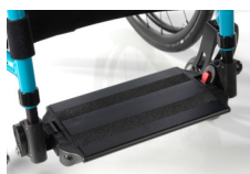
Footboard, angle and depth adjustable; flip up, aluminium with locking system
