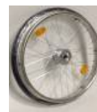
Rear wheel, drum brakes, 36 spokes, cross- wise spokes
