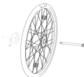
22", 24" rear wheel with drum break, 36 spokes (silver), cross-wise spokes
