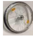
Rear wheel, drum brakes, 36 spokes, cross-wise spokes
