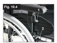
To remove the sideguard completely, push the lever (2). When fitting the sideguard, the lever (2) must also be pulled.
