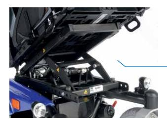
Powered tilt module (0° to 30°) with centre of gravity adjustment to suit correct users balance.
