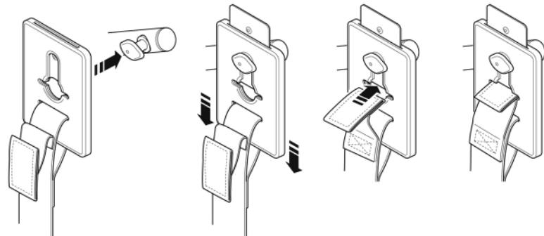
**Securi3 sling attachment system.** Example of installation.
