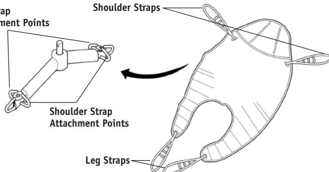
**6 Point spreader bar.** Example of 6 point spreader bar sling with loop attachments.
